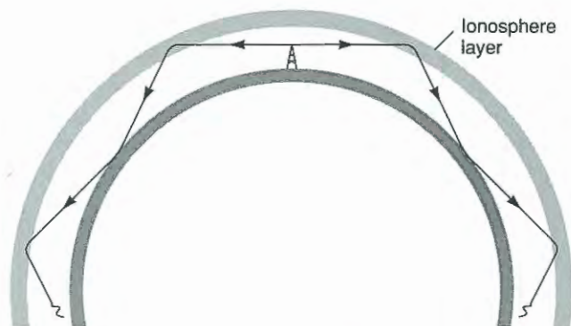
FIGURE 4-1 Skywaves radiate outward above the horizon into space. However, when they encounter the ionosphere, waves of certain frequencies are refracted back toward the earth. The return wave may bounce off the earth back to the ionosphere, then back to earth and so on, in a series of skips. This is the principle of "shortwave" broadcasting.
