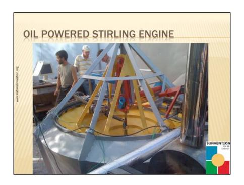
With the cover removed you can see a similar mechanism to the SunPulse Water. This one is using about 7.5kw of heat to generate about 1.5kw (electrical),
