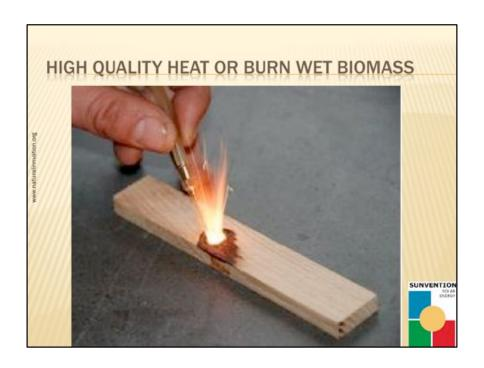
The oxygen can be used either to create a very hot flame – notice the white hot flame from burning ordinary wood here – this is useful for high temperature uses such as ceramics where otherwise you'd use energy expensive fans.
