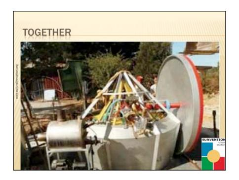
And connecting all the parts together, you also see the flywheel which makes sure the power is the same at each step of the cycle.
